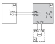
A1: Drive A2: Braking unit A3: Braking resistor PA, DC Bus
